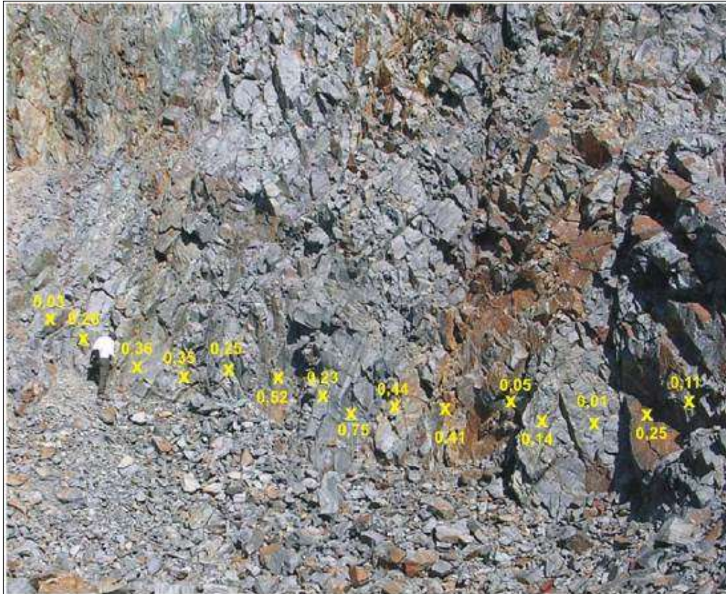
Figure 6-8. Cu Analyses Along lower NE wall at Hovedfelt
