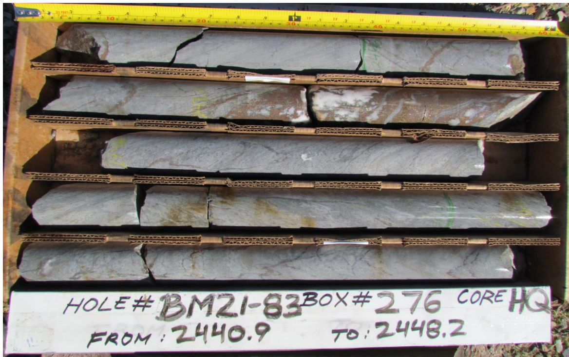
Photo from Mineral zone of BM-83 hole depth 2,440.9 feet. Red brown mineral is sphalerite. Brassy mineral is Chalcopyrite.
