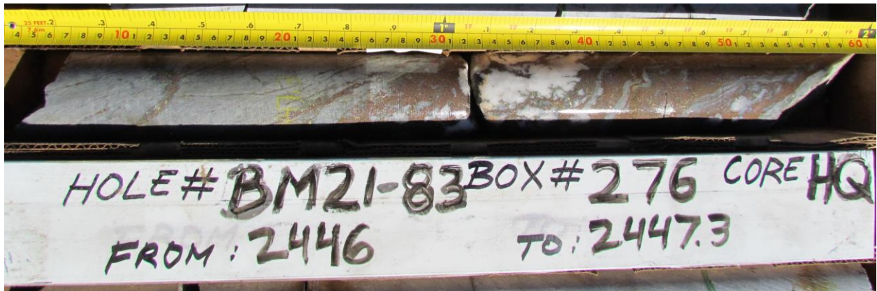
Photo from Mineral zone of BM-83 hole depth 2,440.9 feet. Red brown mineral is sphalerite. Brassy mineral is Chalcopyrite.
