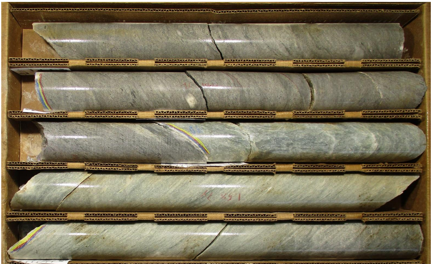
Figure 5: Massive sulphide mineralized interception at hole BMZ80 from 404.52 metres to 407.19 metres downhole depth which includes the highest zinc grade interval returned by this hole, 2.16 metres at 16.49% zinc, 0.89% copper, 0.32% lead, 0.7 g/t gold and 35 g/t silver for a ZnEq of 20.9% from 405.55 metres. Sulphide mineralization mostly follows primary foliation in the hosting rhyolite rock. Sphalerite is pale brown. This photo is of a select sample and not necessarily representative of mineralization hosted on the property.
