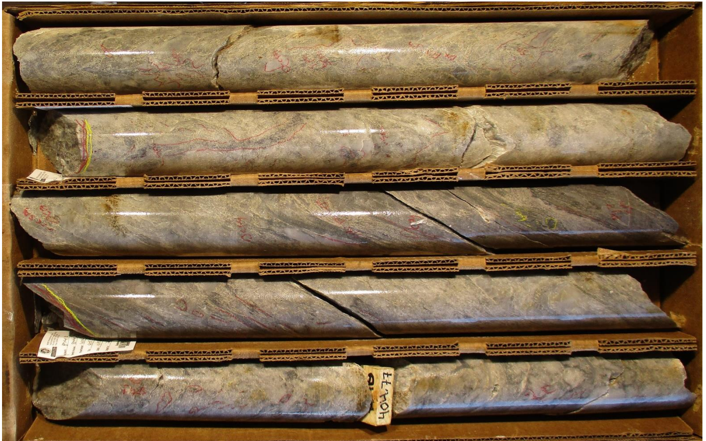
Figure 5: Massive sulphide mineralized interception at hole BMZ80 from 404.52 metres to 407.19 metres downhole depth which includes the highest zinc grade interval returned by this hole, 2.16 metres at 16.49% zinc, 0.89% copper, 0.32% lead, 0.7 g/t gold and 35 g/t silver for a ZnEq of 20.9% from 405.55 metres. Sulphide mineralization mostly follows primary foliation in the hosting rhyolite rock. Sphalerite is pale brown. This photo is of a select sample and not necessarily representative of mineralization hosted on the property.
